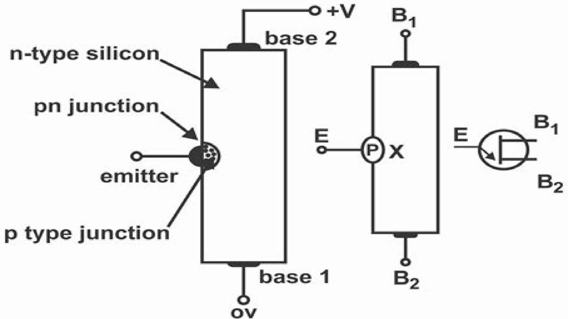
**Fig 7.1 (a) Unijunction transistor
